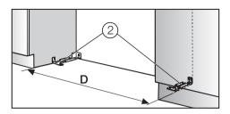
The distance "**D**" between the anti-tip brackets (2) is the width of the appliance.
